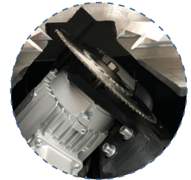
45° main cutting blade & smaller blade to remove the back of each bead
